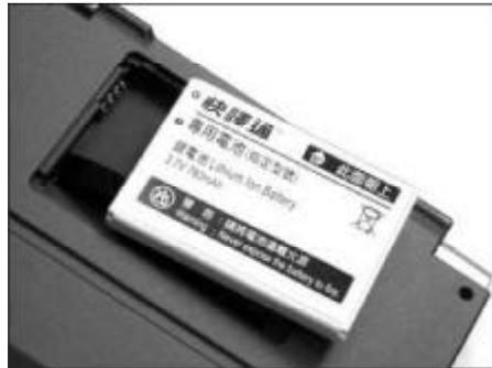
3. Close the batteries compartment door properly.
